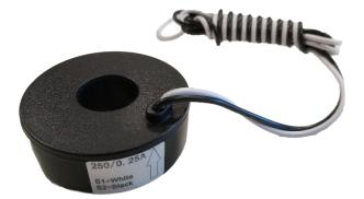
**TRC1 250A transformers** are current transformers specially designed for being installed at the top of a circuit breaker. All the models have secondary of 250 mA and are suitable for SKM8, SKT8 and for third-party devices.
