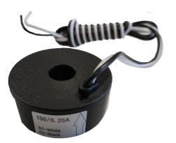
**TRC1 100A transformers** are current transformers specially designed for being installed at the top of a circuit breaker. All the models have secondary of 250 mA and are suitable for SKM8, SKT8 and for third-party devices.
