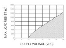
**Supply in AC:** The electronic circuit provides a voltage of 24 VDC to power the loop. The load resistor should not exceed 800 ohms.
