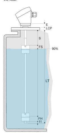
You can determine a bound (S) to establish an area where there is no reading at all. In case you want to remove the head of the connection process (for reasons of high temperature, for example) may specify a dimension (E) exceeding the standard.
