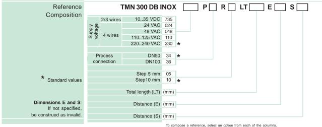
To compose a reference, select an option from each of the columns. Example: TMN 300 DB INOX 230 P34 R10 LT1500 S75
