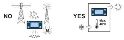
The connections must be done separating, phisically, the measurement signals from the control or power signals.
