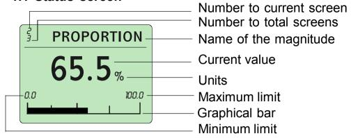
The status screens show the actual values of the magnitudes that the equipment controls . In the normal working mode, the equipment shows the status screen that the user has chosen like preferring magnitude of visualization.
