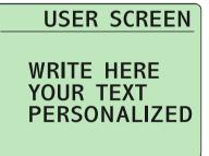
The text edited in the user screen is the one that will be shown next to the status screens when the equipment is i the normal working mode. The characters that can be used are the following:
