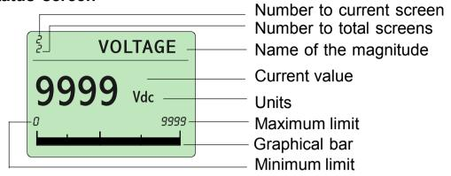
The status screens show the actual values of the magnitudes that the equipment controls. In the normal working mode, the equipment shows the status screen that the user has chosen like preferring magnitude of visualization. In order to move around among the different status screens of status, press  $\blacktriangleright \nabla$ .
