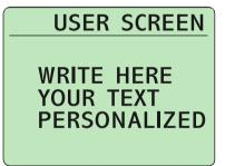
The text edited in the user screen is the one that will be shown next to the status screens when the equipment is in the normal working mode. The characters that can be used are the following:
