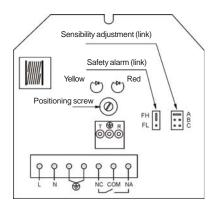
Maximum section of the conductors is to 1.5mm<sup>2</sup>
