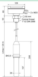
VIBRATING LEVEL SENSOR FOR SOLIDS IN GRAIN. EXTENDED WITH CABLE.
