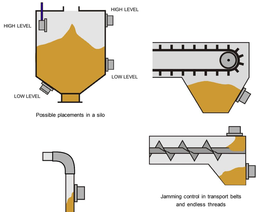
Loading control in pipes working at full tube.
