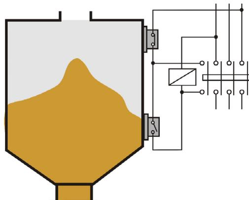
Schematic for an automatic control according to the level changes of the material in a silo.
