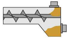
Jamming control in transport belts and endless threads
