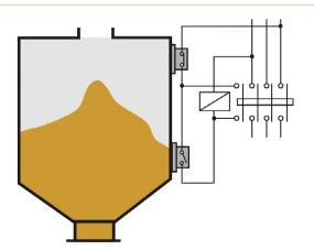
Schematic for an automatic control according to the level changes of the material in a silo.
